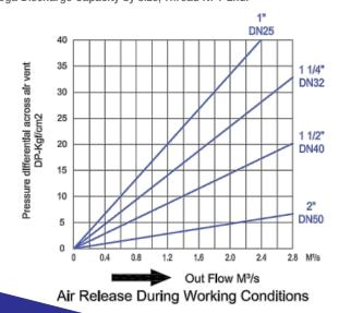
Omega Vacuum flow Charge Capacity by size, Thread NPT End:
