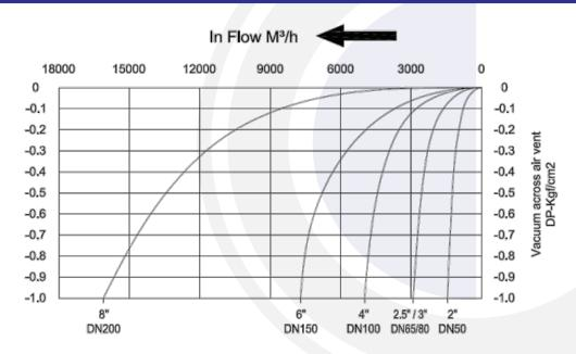
Omega Discharge Capacity by size, Thread NPT End:
